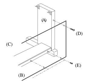
2. Fasten Side Panel (A) and Back Panel (B) with two screws (D). Then fix Back Panel (B) to Pedal Board (C) with four screws (E).
